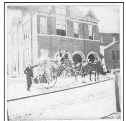
Photo from the Fred A. Grier Collection of a Silsby Steamer bought in 1879 by the Salisbury Fire Department. In 1900 the metal wheels were changed to wood.
