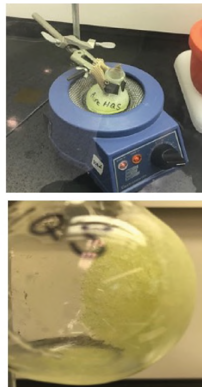
Figure 4: HQS purification. Set-up of heating HQS to a boil during purification in acidic conditions. Purified crystals. Images courtesy of Thomas Montag.
