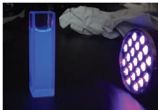
Figure 5: Carbon quantum dots made from sodium citrate.
