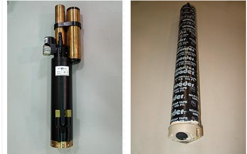
Water Quality Monitor (left) and Acoustic Current Profiler (right)
